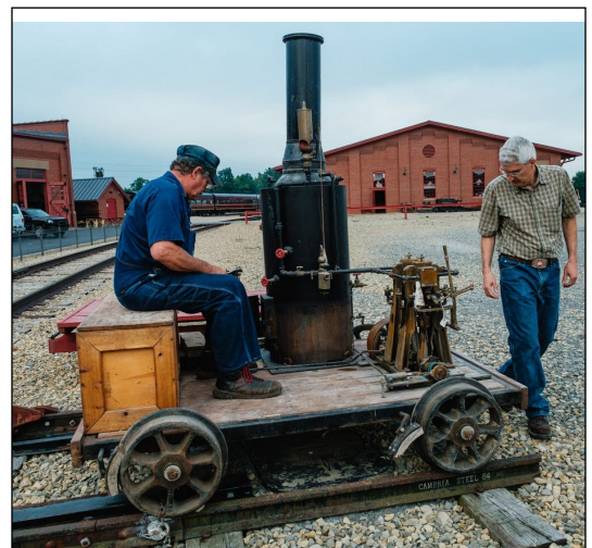
Above is a photo of a steam powered speeder. How is that for combining steam and vehicles in one photo?
