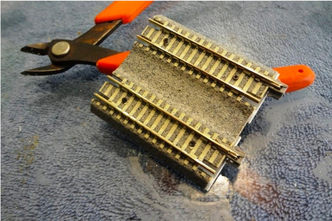
In Photo 3, you see one of the completed alignment jigs. I built a second one following the same steps so I could align both ends of the track at the same time. The styrene strips, which extend 1mm beyond the end of the track, are apparent underneath, as are the screws that are holding the strips in place.
